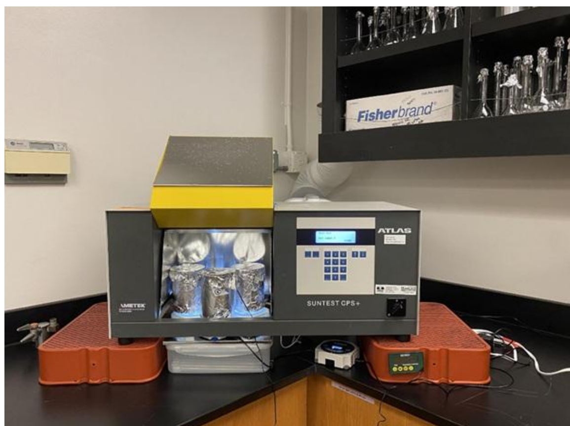
Figure 3: Leachate setup in the Atlas Suntest CPS+ photoradiation machine.
